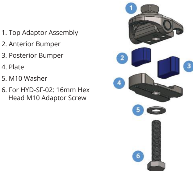
Fig. 8 Adjustable Stance Flexion Adaptor Assembly
